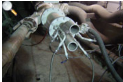
A burner for petcoke, solid wastes (two channels), liquid wastes/heavy fuel oil ( http://www.dynamis-ma.com/ ).
