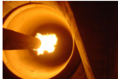
Burner for petcoke, solid wastes, natural gas / diesel oil lance. ( http://www.dynamis-ma.com/ )
