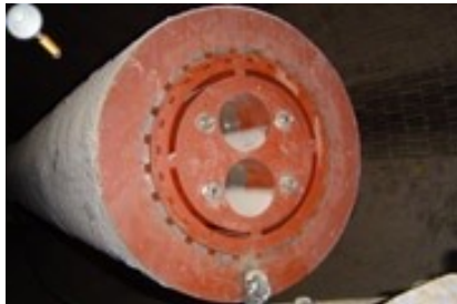
A burner for petcoke, solid wastes (two channels), liquid wastes/heavy fuel oil ( http://www.dynamis-ma.com/ ).
